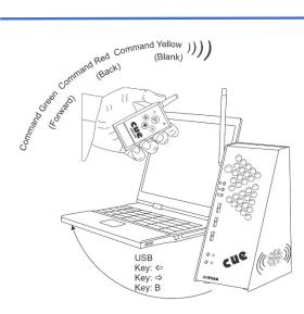
Keystroke commands that control presentations are stored in the base cue light. There is a separate keystroke —or keystroke macro — for each button on the transmitter.
